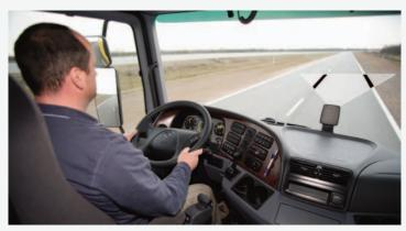
close to the vehicle in front, applying the brakes and retarder, if necessary, to keep the speed relative to the traffic ahead, ACC is designed to reduce stress for the driver on longer hauls.
